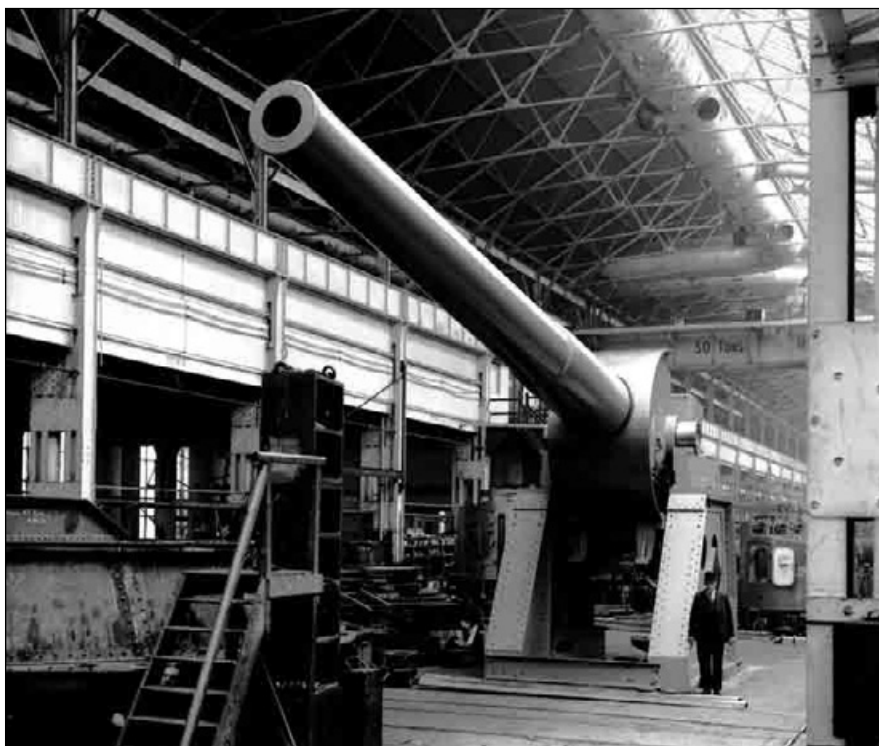
20. Unknowingly preparing to fight the next war but one: a fifteen-inch naval gun being made by Vickers before the Great War. More than 180 were produced for British battleships. Most were still in service in the Second World War, where they found more use than in the Great War.
