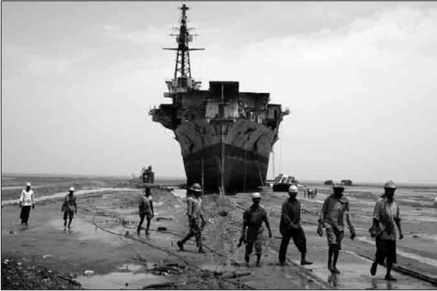
27. The Brazilian aircraft carrier Minas Gerais, broken up with a novel lack of modern technology on Alang Beach, Gujarat, India, in 2004. Alang Beach became the single largest centre of the shipbreaking industry, and a startling example of the new technological retrogression. The ship, originally HMS Vengeance, launched in 1945, was built at a time when shipbreaking was more capital intensive.
